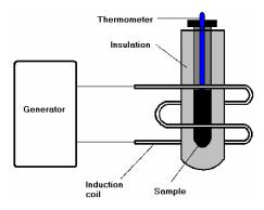
Fig. 1. The sketch of the experimental device. The sample was put in an field created by an induction coil conected to a AC power source. The temperature was measured with an alcohol thermometer through direct reading.
