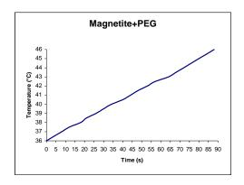
Figure 2. Temperature evolution ( $^{\circ}C$ ) depending on time (s) in colloid I.
