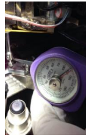
b. Correx hand held bond force gauge to confirm the DA force on DA equipment.
