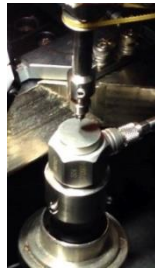
a. Keyence - Compression Load Cells installed on DA equipment
