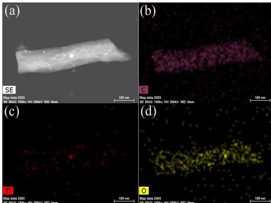
Fig. 3 (a) TEM of EDS mapping of selected area, (b) element C mapping, (c) element Ti mapping, (d) element O mapping of G/PCF/TiO<sub>2</sub>
