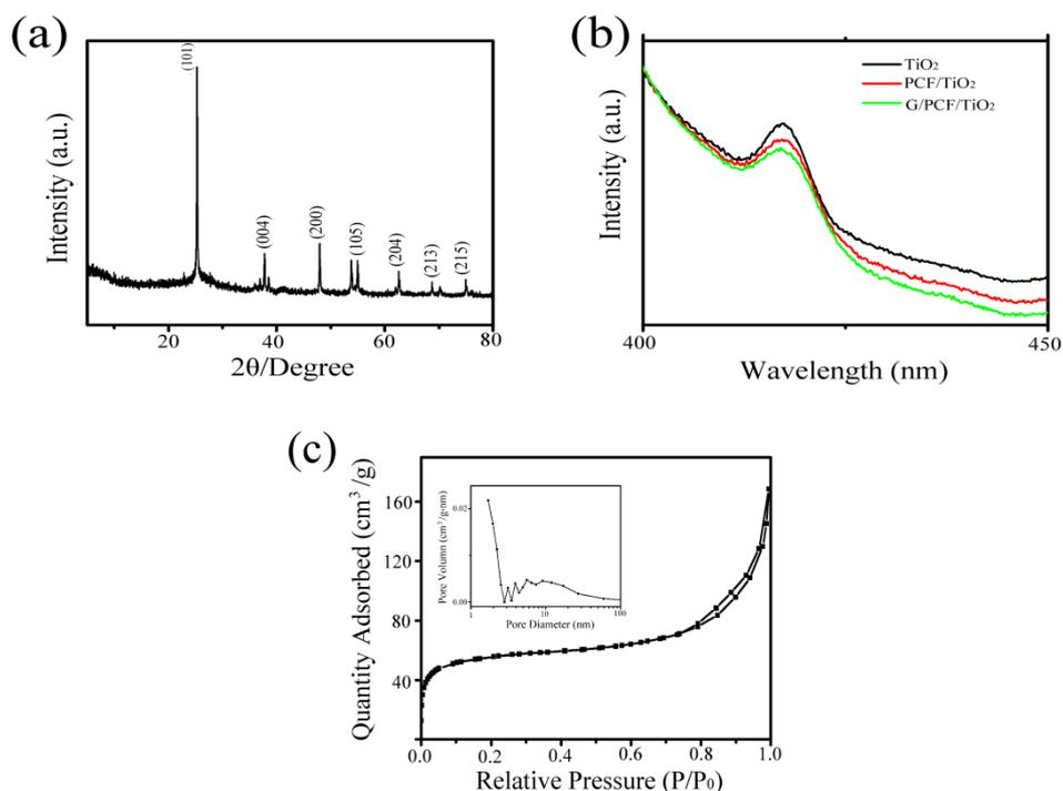
Fig. 4. (a) XRD, (b) photoluminescence spectra, (c) nitrogen adsorption/desorption isotherms and pore size distribution of the samples.
