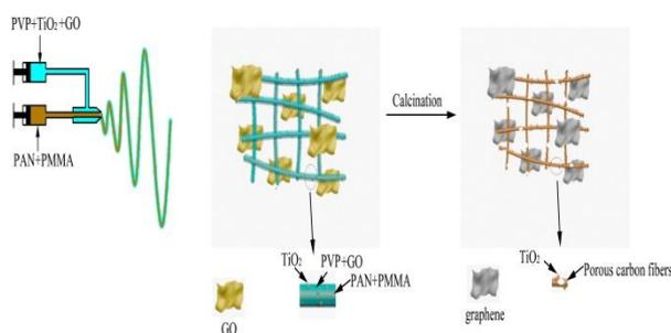
Fig. 1. Schematic illustration of the co-axial electrospinning and carbonization processes.
