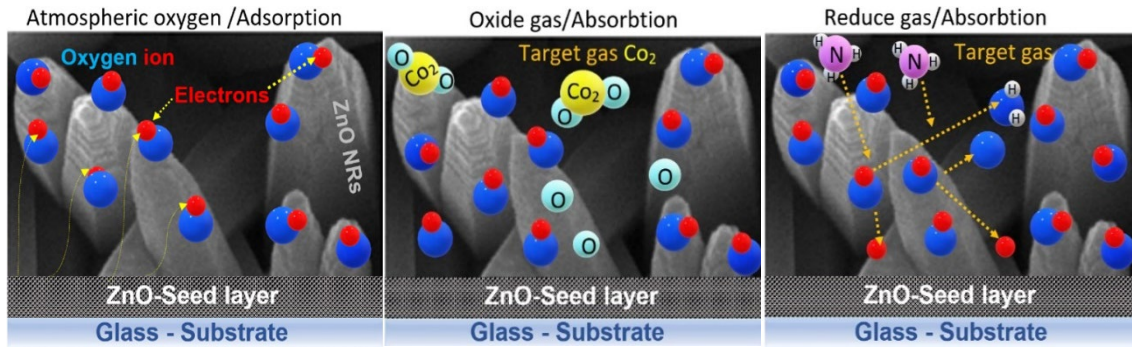
Fig. 4. Sensing mechanism (adsorption, absorption of oxide and reduced gas) of ZnO NRs.
