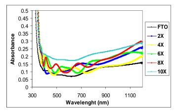
Fig. 3. The absorption spectra of the spin-coated TiO<sub>2</sub> buffer layers of various thicknesses, compared to the bare FTO glass.
