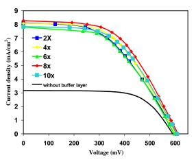
Fig. 10 Current-voltage curves for typical dye-sensitized solar cells fabricated with T2X (square), T4X (diamond), T6X (triangle), T8X (gray circle), T10X (empty circle) and without buffer layer (line) photoelectrodes
