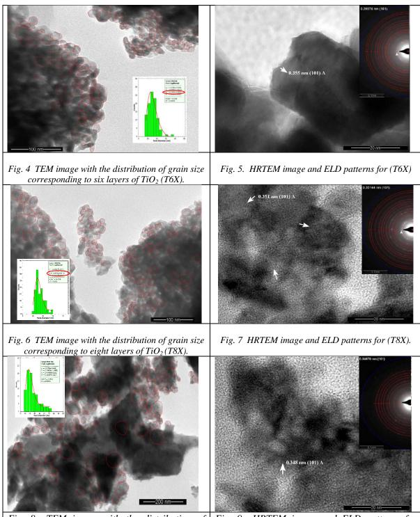
Fig. 8 TEM image with the distribution of Fig. 9 HRTEM image and ELD patterns for grain size corresponding to eight layers of  $TiO_2$  (T10X).
