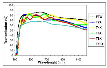
Fig. 2. The transmission spectra of the spin-coated TiO<sub>2</sub> buffer layers of various thicknesses, compared to the bare FTO glass.
