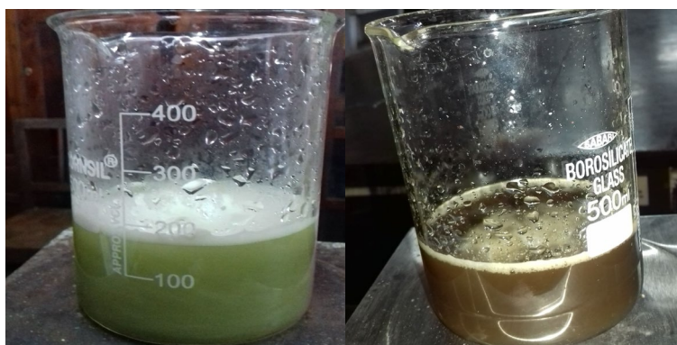
Fig. 2. Green fabrication of CuNPs using the Andrographis leaf extract and copper sulphate.
