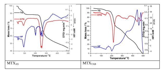
Fig. 2. The thermoanalytical curves TG/DTG/HF obtained in air at  $\beta=10$  °C·min<sup>-1</sup> for the analysed samples.
