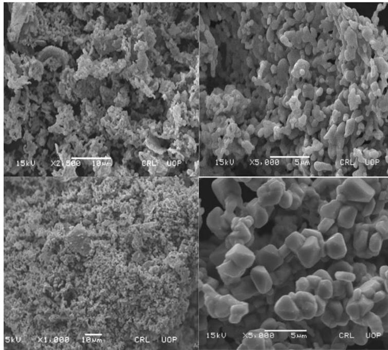
Fig.5. FESEM images of the w type hexaferrites  $Sr_{1-x}Cr_xCo_2Fe_{16}O_{27}$  with ( $x=0.4,0.6,0.8,1.00$ ).
