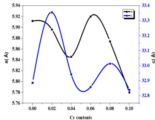
Fig. 2. Lattice constant  $a$  and  $c$  of the  $\text{Sr}_{1-x}\text{Cr}_x\text{Co}_2\text{Fe}_{16}\text{O}_{27}$  ( $x=0.0, 0.02, 0.04, 0.06, 0.08, 0.1$ ) hexaferrite magnetic powders.
