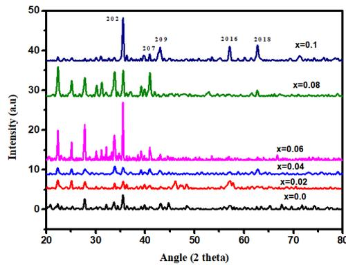
Fig. 1. XRD pattern of W type Sr<sub>1-x</sub>Cr<sub>x</sub>Co<sub>2</sub>Fe<sub>16</sub>O<sub>27</sub>(x= 0.0, 0.02, 0.04, 0.06, 0.08, 0.1) hexaferrites.
