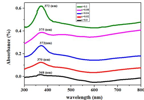
Fig. 4. UV-VIS Analysis of  $Sr_{1-x}Cr_xCo_2Fe_{16}O_{27}$  hexagonal ferrite at  $x=0$ ,  $x=0.02$ ,  $x=0.04$ ,  $0.08$ ,  $x=0.1$ .
