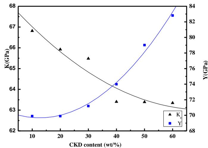
Fig. 3: Variation of elastic moduli versus CKD wt. %
