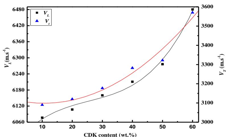
Fig. 2: Variation of ultrasonic velocity versus CKD wt. %
