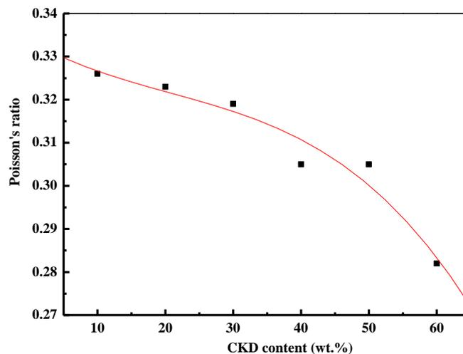
Fig. 4: Variation of Poisson's ratio versus CKD wt. %
