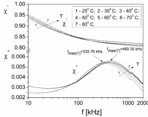
Fig. 2a. The frequency and temperature dependencies of the ( $\chi'$ ) and ( $\chi''$ ) components of the complex dielectric susceptibility.
