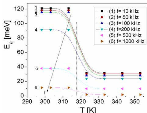
Fig. 4. The dependence on temperature of the activation energy  $E_a$  for different frequencies  $f$ .
