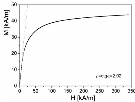
Fig. 1. Magnetization curve for investigated ferrofluid.
