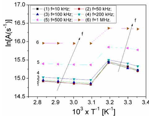
Fig. 3. The dependence of  $\ln(A)$  on  $(1/T)$  at different frequency  $f$ , for the ferrofluid sample.
