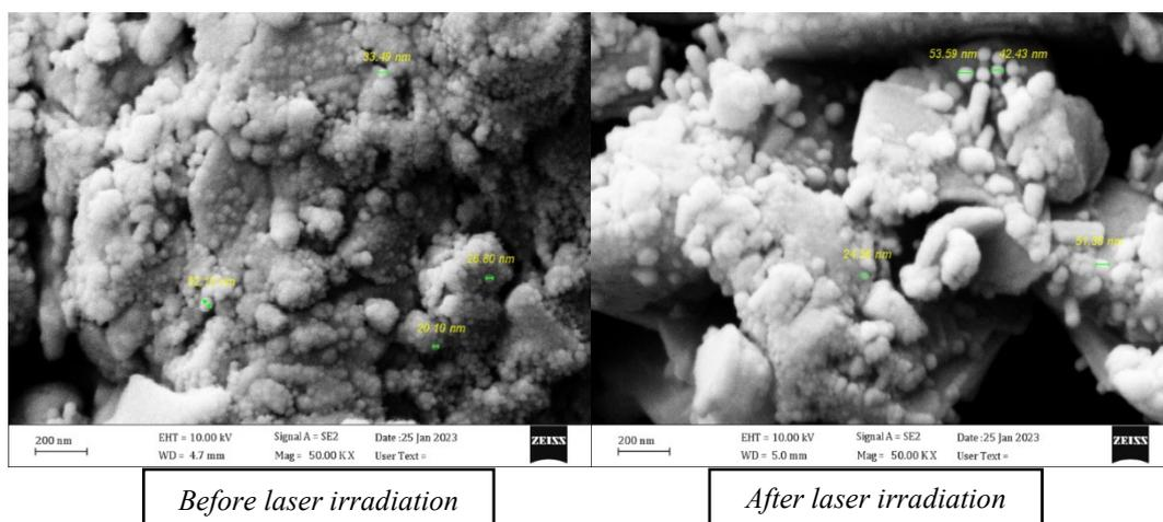
Fig. 4. FESEM for nanocomposite  $\text{Bi}_2\text{Sr}_{2-x}\text{Y}_x\text{Ca}_2\text{Cu}_{3-y}\text{Ni}_y\text{O}_{10+\delta}$  specimen B, before and after laser irradiation where  $x=0.03$ ,  $y=0.03$ .
