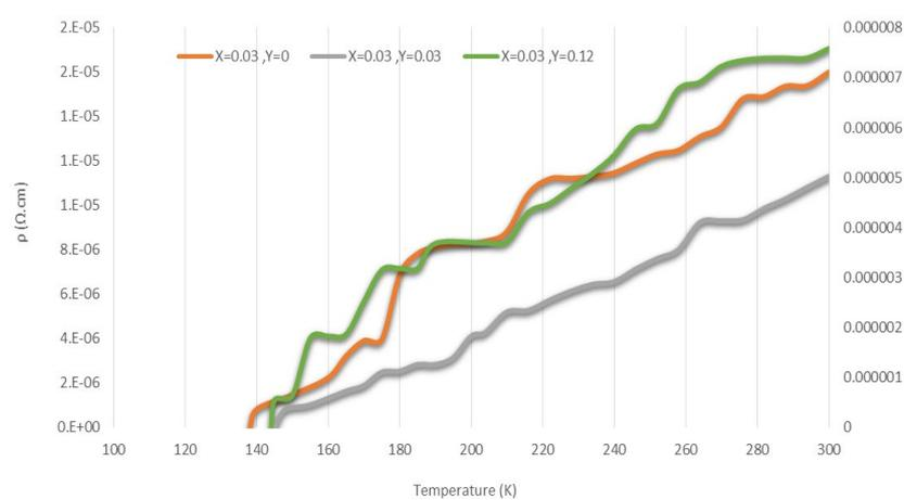
Fig. 3. The relationship between temperature and electrical resistivity for  $\text{Bi}_2\text{Sr}_{2-x}\text{Y}_x\text{Ca}_2\text{Cu}_{3-y}\text{Ni}_y\text{O}_{10+\delta}$  after laser irradiation.
