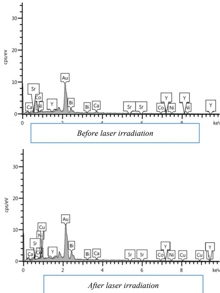
Fig. 5. EDS image of nanocomposite  $\text{Bi}_2\text{Sr}_{2-x}\text{Y}_x\text{Ca}_2\text{Cu}_{3-y}\text{Ni}_y\text{O}_{10+\delta}$  specimen B, before and after laser irradiation where  $x=0.03$ ,  $y=0.03$ .
