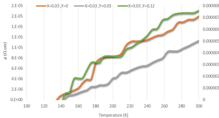
Fig. 2. The relationship between temperature and electrical resistivity for  $\text{Bi}_2\text{Sr}_{2-x}\text{Y}_x\text{Ca}_2\text{Cu}_{3-y}\text{Ni}_y\text{O}_{10+\delta}$ , before laser irradiation.
