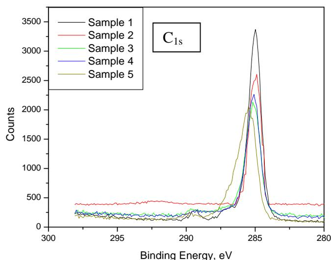
Fig. 7 XPS spectra of the carbon on the worn surface
