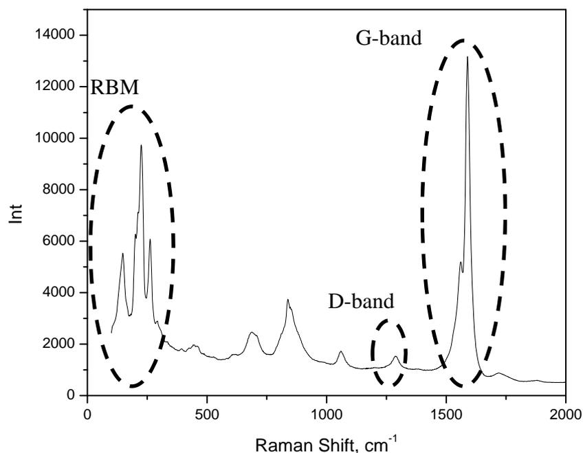
Fig. 1 Raman shift recorded after SWNT growth (at 785 nm wavelength)
