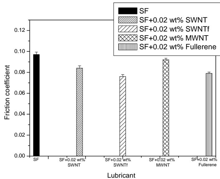
Fig. 4 Friction coefficients of vegetable oil with different carbon nanomaterials such antiwear additives
