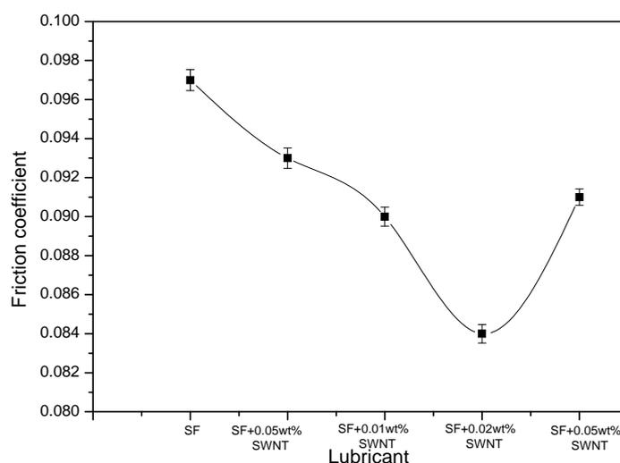
Fig. 3 Friction coefficients for vegetable oil with different SWNTs concentrations
