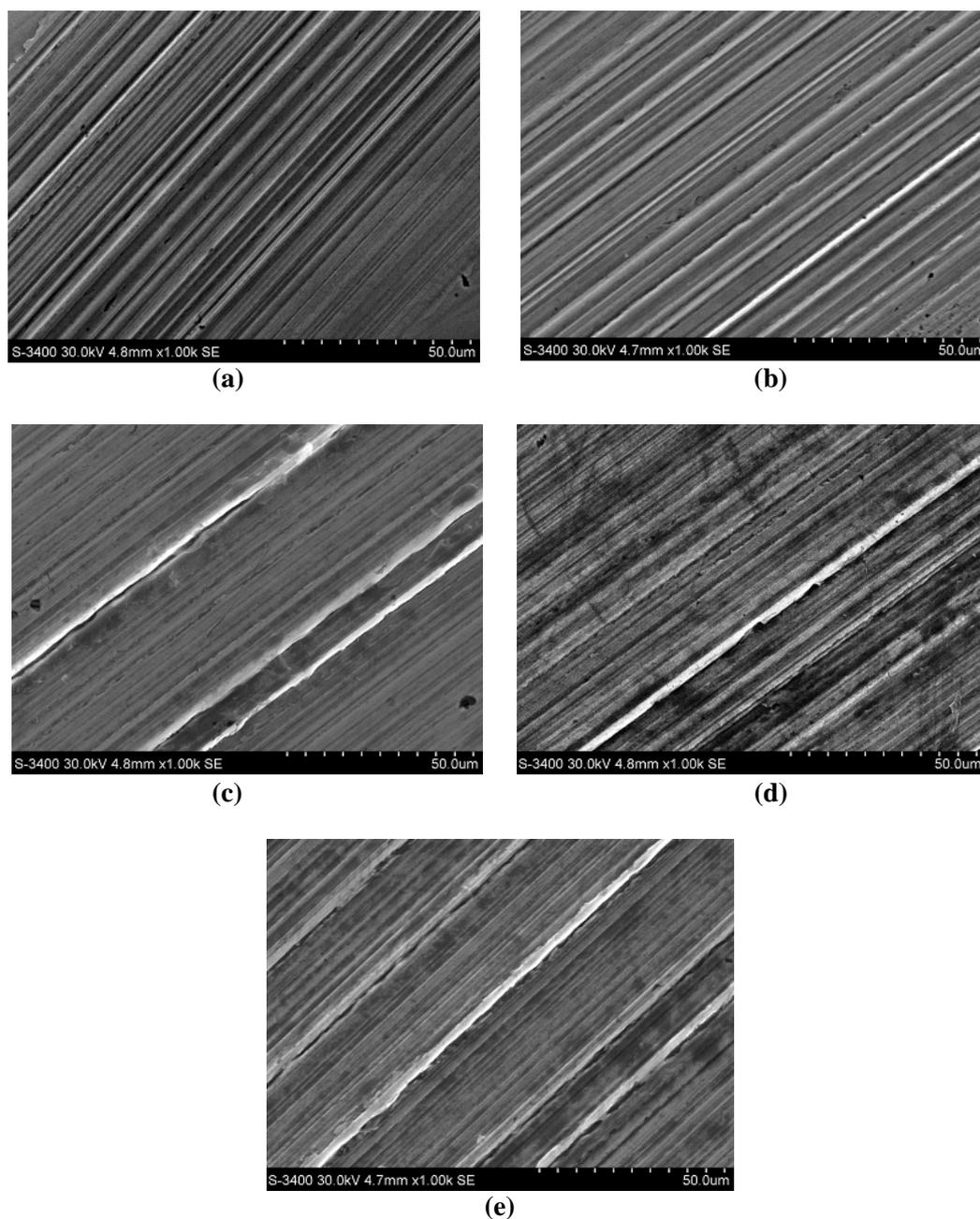
*Fig. 5 SEM images of the friction surface of the disk after the friction test*
