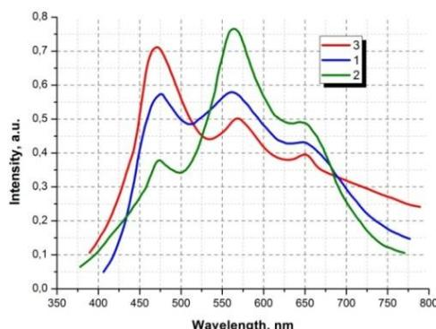
Figure 5. The PL spectra of ZnS-PS structure at different molar concentration of initial components of solution.
