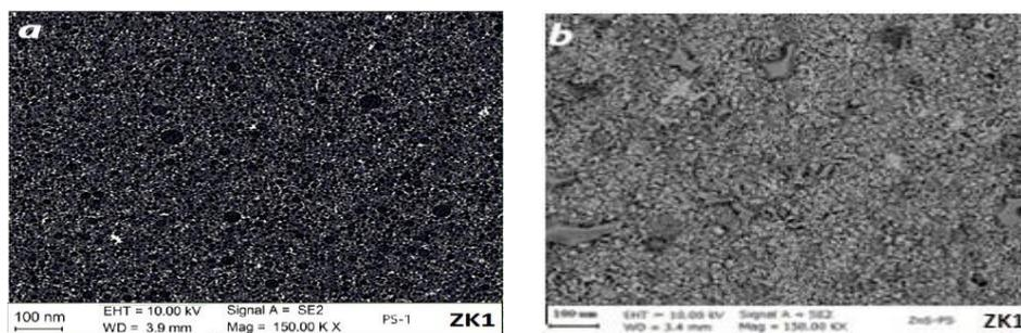
Figure 2. SEM images of the surface of porous silicon with a pore size of 10–15 nm (a), and the surface after deposition of ZnS into PS (b).
