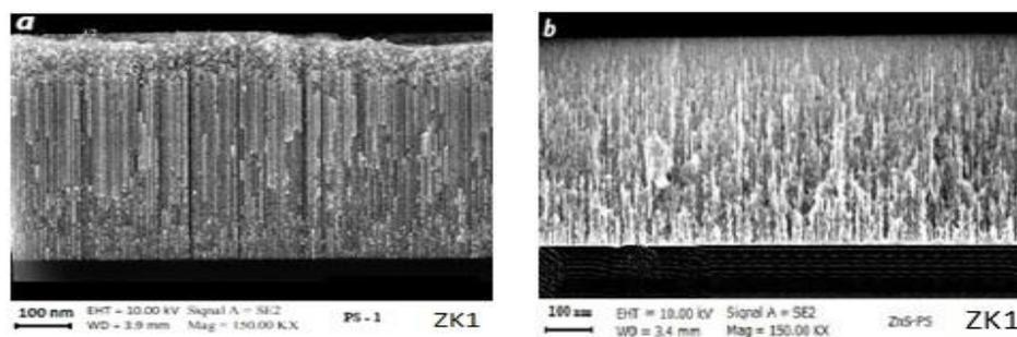
Figure 3. SEM image of a cross section of a silicon wafer etched for 30 min (a) and after deposition of ZnS particles (b).
