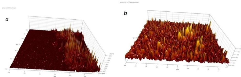
Figure 1. AFM images of the surface of PS with pore size of 10–15 nm (a), and the surface after deposition of ZnS into PS (b).
