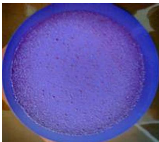
Fig. 5. Membrane filter assay for detection of E-coli in the water sample before filtration. The approximate number of bacteria is 1000cfu/mL.
