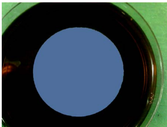
Fig. 9. Membrane filter assay for detection of E-coli in the treated water sample after 6.5h filtration. There is no bacterium in this image.
