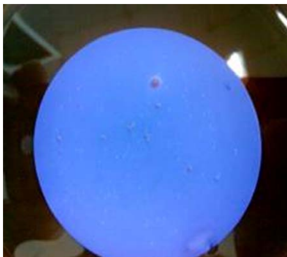
Fig. 8. Membrane filter assay of 45nm nano silver-coated filter for detection of E-coli in the treated water sample after 6 hours filtration.
