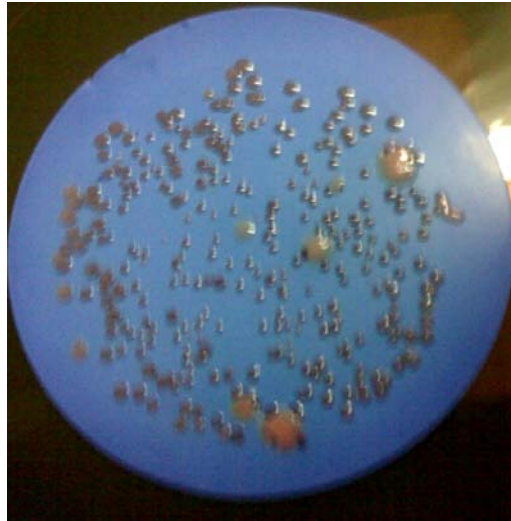
Fig. 6. Membrane filter assay of 45nm nano silver-coated filter for detection of E-coli in the treated water sample after 2 hours filtration. The number of bacteria is equal to 486cfu/mL.
