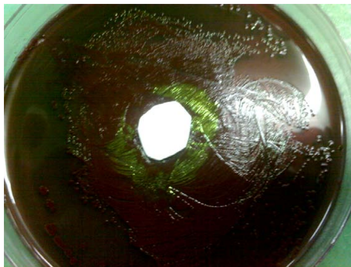
Fig. 12. Zone of inhibition test result of the uncoated polypropylene water filter for E. coli with nutrient agar plating.
