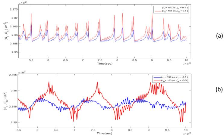
Fig. 4. Photon density with time for Transmitter and Receiver laser of (QDSL) when  $(\tau_T = 150 \text{ ps}, \tau_R = 155 \text{ ps})$  for (a): positive and (b): negative optoelectronics feedback.
