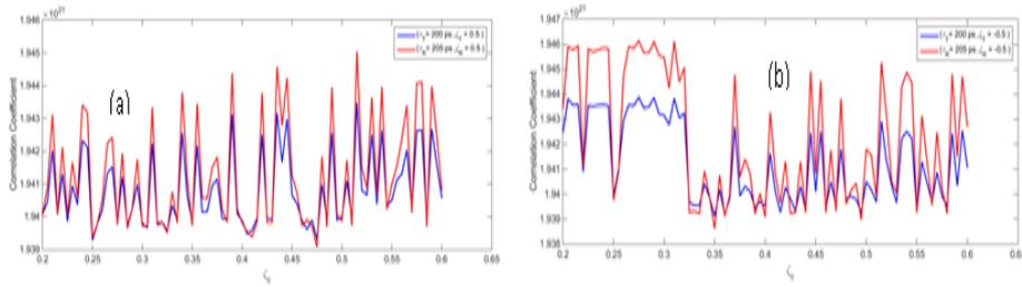
Fig. 5. Correlation Coefficient and Photon density as a function of ( $\zeta_c$ , time) of (QDSL) when ( $\tau_T = 200 \text{ ps}, \tau_R = 205 \text{ ps}$ ) with (a) : positive and (b) :negative optoelectronics feedback.
