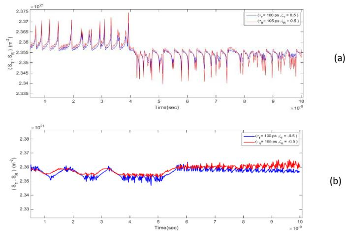
Fig. 2. Photon density with time for Transmitter and Receiver laser of (QDSL) when ( $\tau_T = 100 ps, \tau_R = 105 ps$ ) for (a) : positive and (b) :negative optoelectronics feedback.
