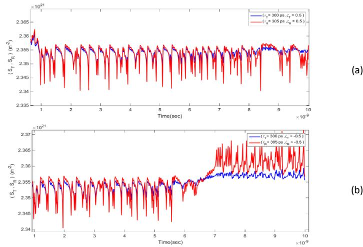
Fig. 8. Photon density with time of transmitter and receiver laser of (QDSL) when  $(\tau_T = 300 \text{ ps}, \tau_R = 305 \text{ ps})$  for (a): positive and (b): negative optoelectronic feedback.
