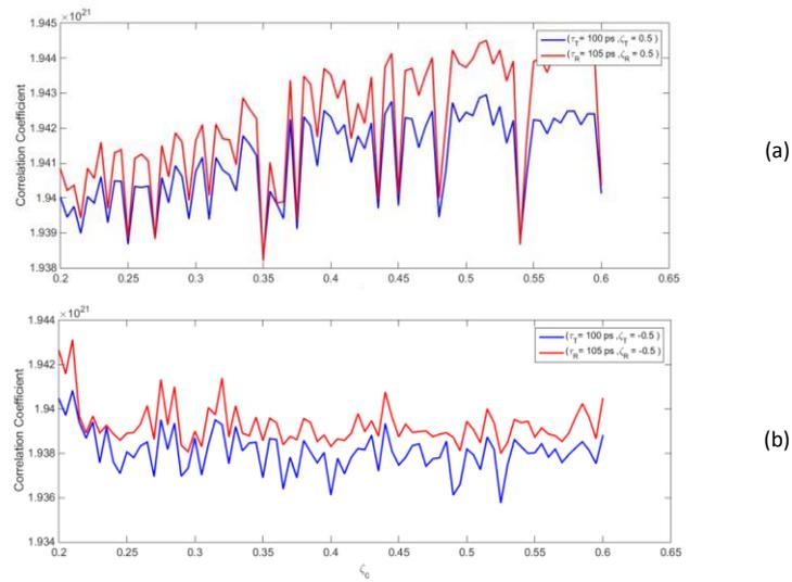
Fig. 1. Correlation Coefficient as a function of ( $\zeta_c$ ) of (QDSL) when ( $\tau_T = 100 ps, \tau_R = 105 ps$ ) with (a): positive and (b): negative optoelectronics feedback.
