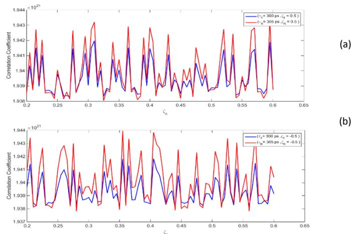
Fig. 7. Correlation Coefficient and Photon density as a function of ( $\zeta_c$ , time) of (QDSL) when ( $\tau_T = 300 \text{ ps}, \tau_R = 305 \text{ ps}$ ) with (a) : positive and (b) :negative optoelectronics feedback.
