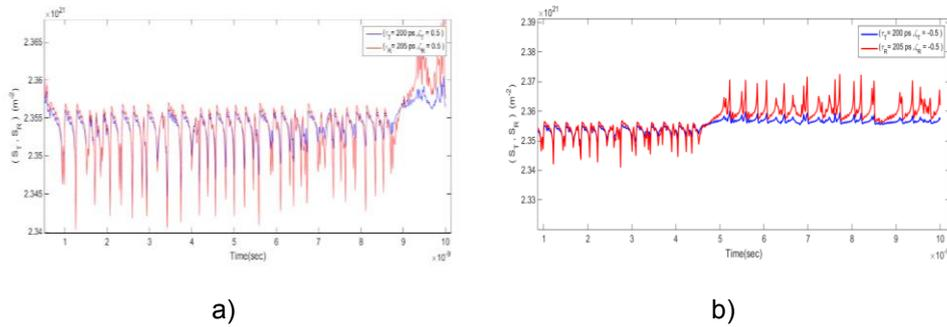
Fig. 6. For photon density with time of transmitter and receiver laser of (QDSL) when ( $\tau_T = 200 \text{ ps}, \tau_R = 205 \text{ ps}$ ) for (a) : positive and (b) :negative optoelectronics feedback.
