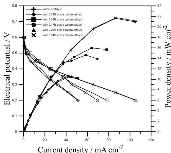
Fig. 6 Power densities of DMFCs with different percentages of active carbon catalyst added onto the channels at an operating temperature of 70°C.
