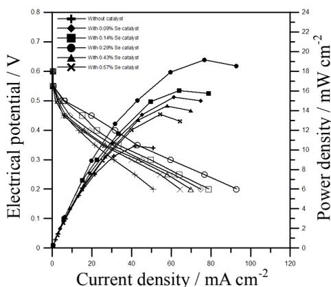
Fig. 7 Power densities of DMFCs with different loadings of Se catalyst added onto the channels at an operating temperature of 70 °C.
