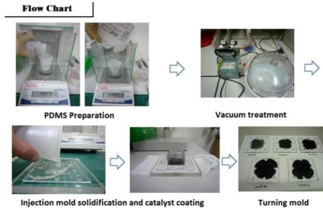
Fig. 1 Injection-molding processes of channel fabrication (Yarn et al. [20]).
