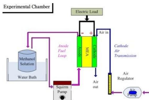
Fig. 4 Schematic diagram of experimental apparatus (Yeh et al. [20]).
