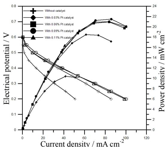
Fig. 5 Power densities of DMFCs with different percentages of Pt catalyst added onto the channels at an operating temperature of 70°C.
