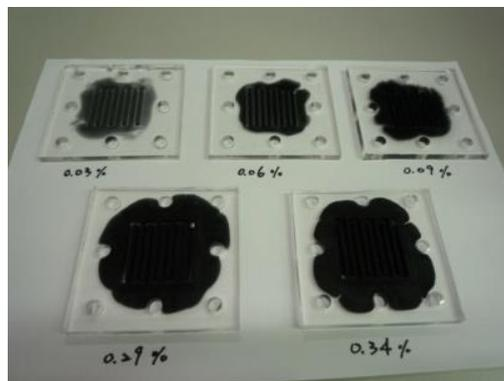
Fig. 2 Channels with different concentrations of active carbon catalyst (Yarn et al. [20]).
