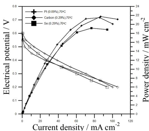
Fig. 8 Comparison of power densities of DMFCs with corresponding threshold percentage values of catalysts added onto the fuel channels at an operating temperature of 70 °C.
