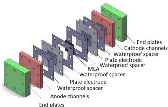
Fig. 3 Exploded view of the transparent DMFC test fixture (Yeh et al. [20]).
