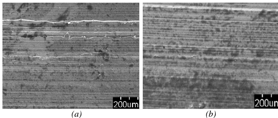
Fig. 5. SEM on the selected typical friction lubricated by (a) base oil and (b) base oil with 1.0 wt% MoSe<sub>2</sub>/MoO<sub>x</sub> at 300rpm.
