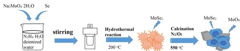
Fig. 1. Schematic diagram of the preparation of heterogeneous  $\text{MoSe}_2/\text{MoO}_x$  nanostructure.
