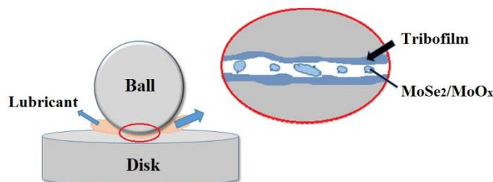
Fig. 6. Schematic diagram of friction reducing and antiwear properties between friction surfaces in the base oil with  $\text{MoSe}_2/\text{MoO}_x$  heterogeneous nanostructures.
