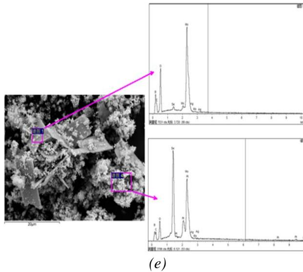
Fig. 2. (a) XRD pattern, (b)(c)(d) SEM image and (e) EDS of the as-obtained MoSe<sub>2</sub>.
