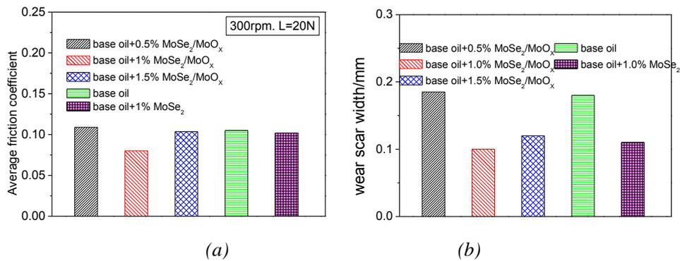
Fig. 3. Variation in tribological properties with increased content of MoSe<sub>2</sub>/MoO<sub>x</sub> in base oil: (a) friction-time curves and (b) average wear scar diameter.
