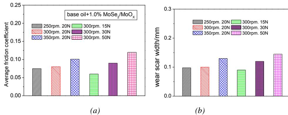
Fig. 4. Variation in the tribological properties of 1.0% MoSe<sub>2</sub>/MoO<sub>x</sub> in base oil with increased load and sliding velocity: (a) friction–time curves and (b) average wear scar width.
