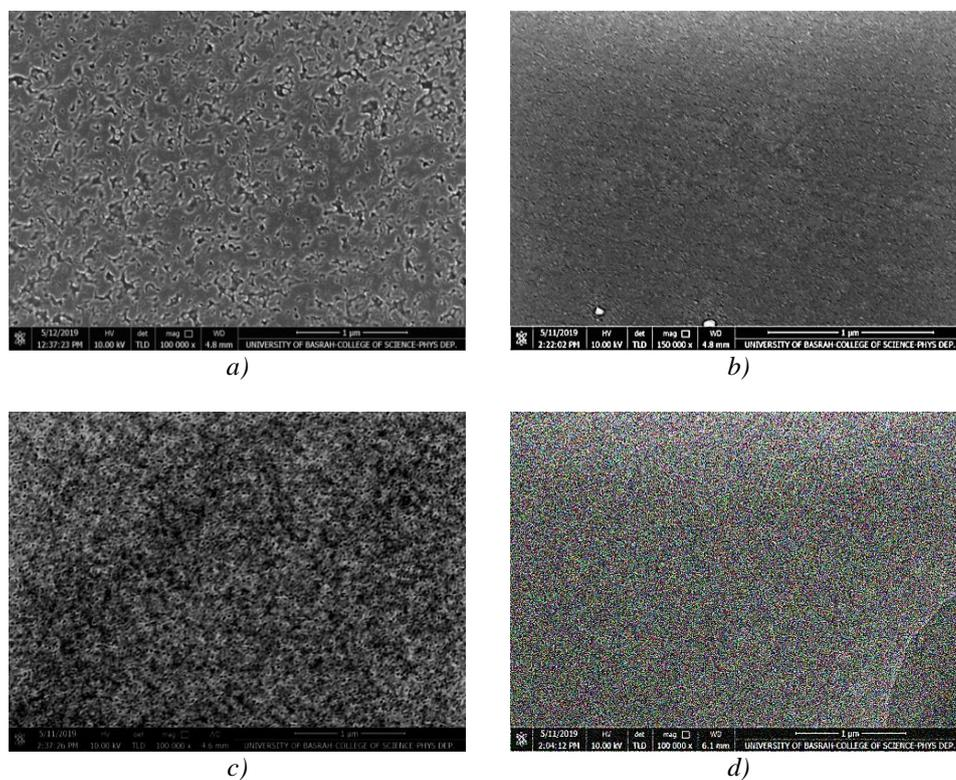
Fig. 2. FESEM image of GaN thin films deposited with different number of coatings onto (a) silicon 3 layers, (b) quartz 3 layers, (c) silicon 7 layers, and (d) quartz 7 layers.
