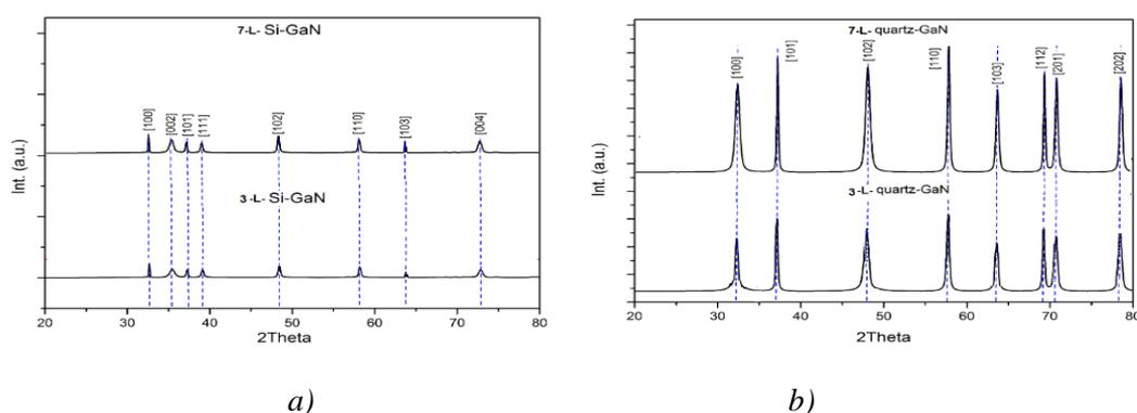
Fig. 1. XRD pattern of GaN thin films deposited with different number of coatings layers onto (a) silicon 7 and 3 layers, (b) quartz 7 and 3 layers.
