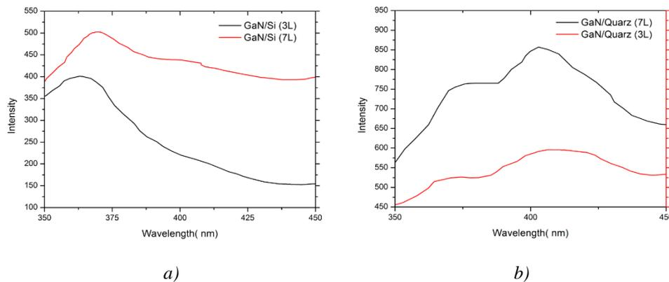
Fig. 3. PL of GaN thin films deposited with different number of coatings onto (a) silicon 7 and 3 layers, (b) quartz 7 and 3 layers.
