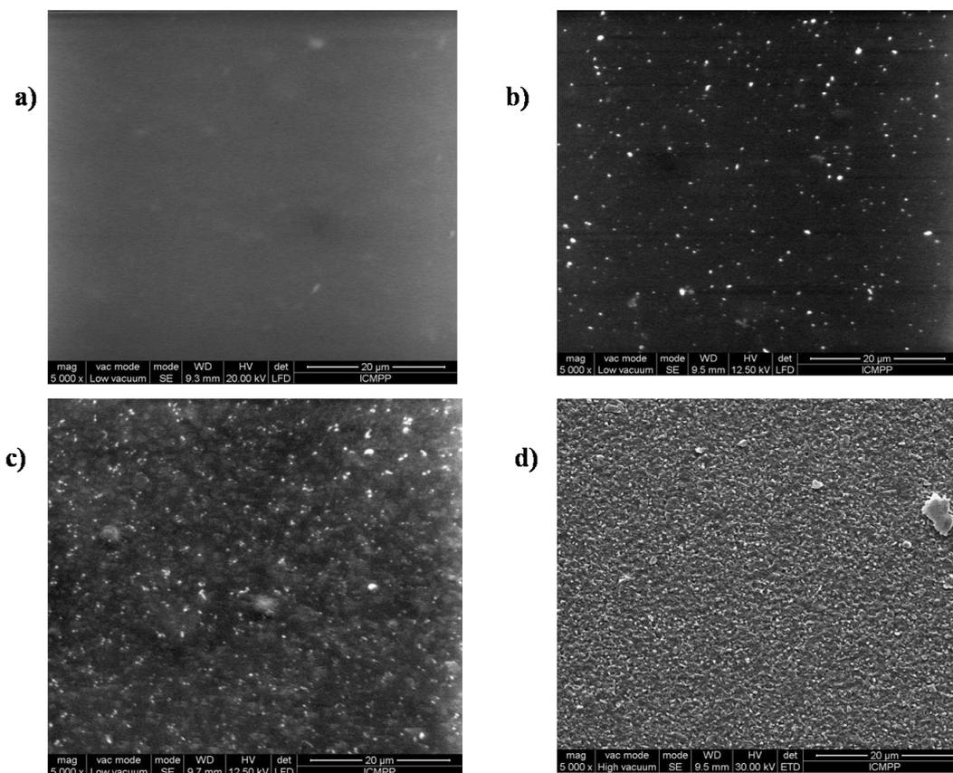
Fig. 1. SEM images for: the untreated PET film (a.); PET 2h UV (b.); PET 50 W, 3 min plasma (c.); PET 50 W, 3min plasma and 2h UV (d.).
