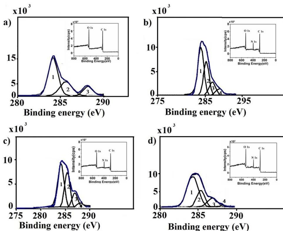
Fig. 3. XPS wide spectra and C1s high resolution spectra of: a) untreated PET; b) PET 2h UV; c) PET 50W, 3min plasma; d) PET 50W 3 min plasma and 2h UV.
