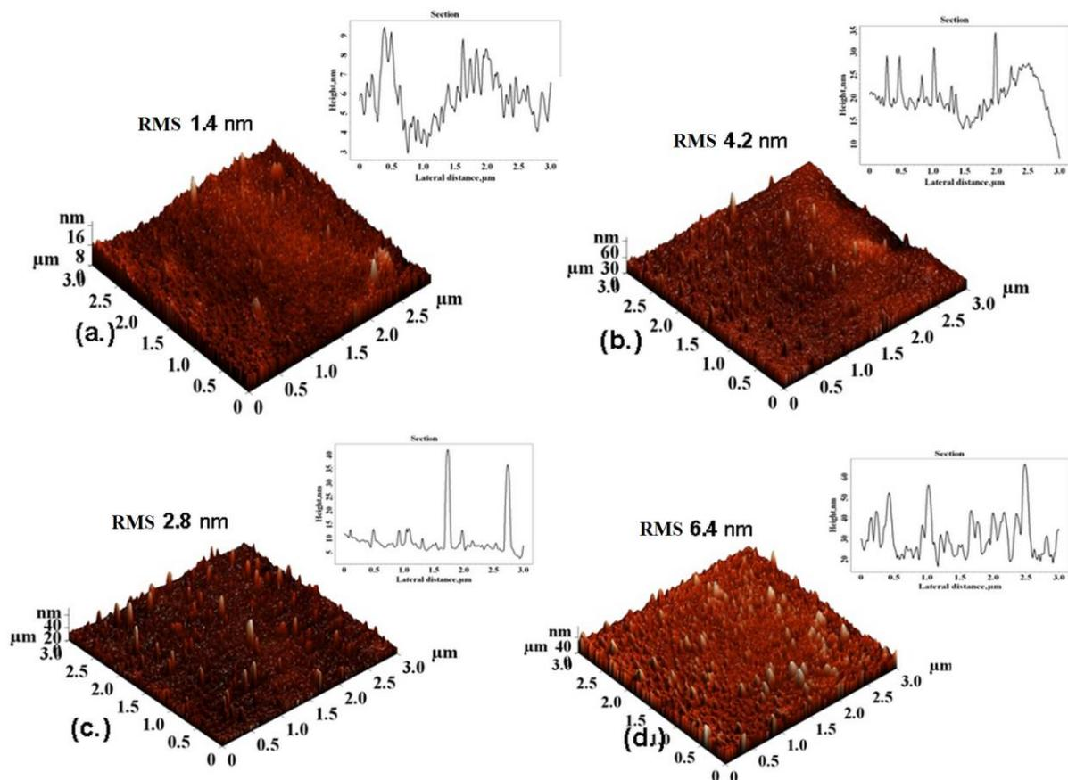
Fig. 2. 3D AFM images for: the untreated PET film (a.); PET 2h UV (b.); PET 50 W, 3 min plasma (c.); PET 50 W, 3min plasma and 2h UV (d.).
