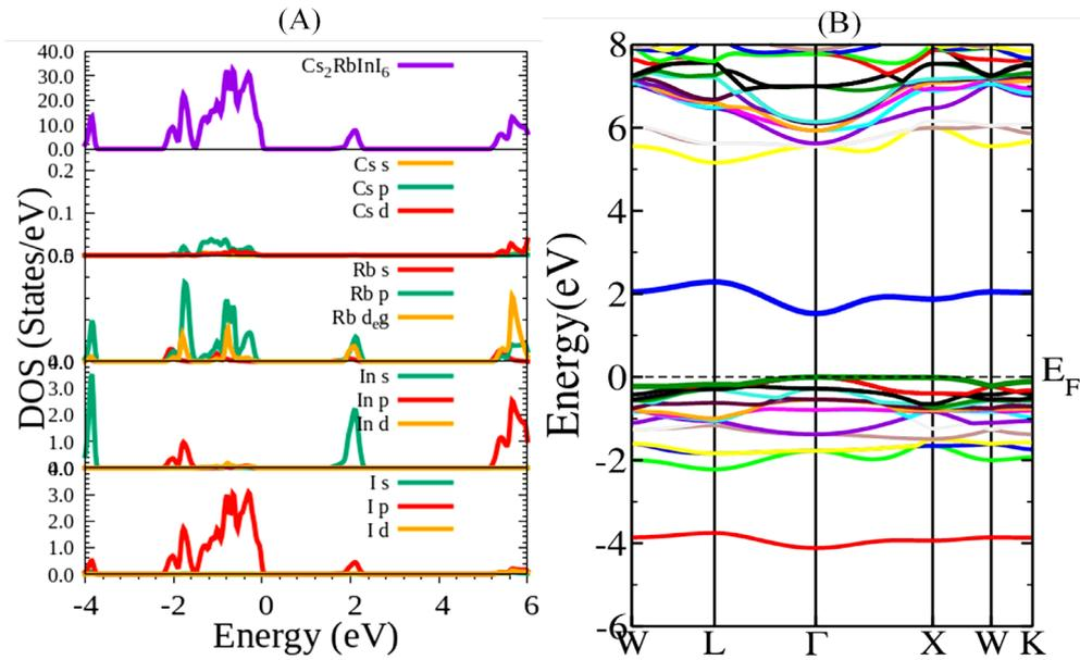
Fig. 2. (A) Total density of states for  $\text{Cs}_2\text{RbInI}_6$  with projectile density of states corresponding to orbitals associated with conduction band minima and valence band maxima, (B) Dispersion curve for  $\text{Cs}_2\text{RbInI}_6$  where  $E_F$  is Fermi energy level.
