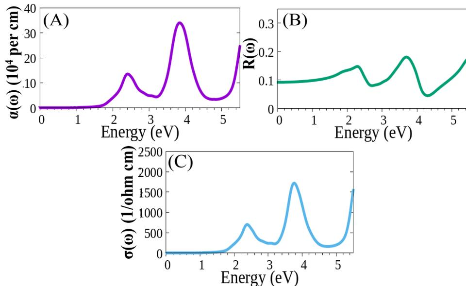
Fig. 3. Dependency of (A) absorption coefficient  $\alpha(\omega)$ , (B) reflectivity  $R(\omega)$  and (C) optical conductivity  $\sigma(\omega)$  on energy for  $\text{Cs}_2\text{RbInI}_6$ .
