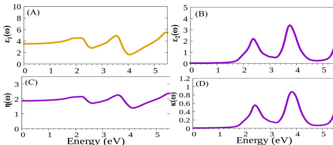
Fig. 4. Real  $\epsilon_1(\omega)$  and imaginary  $\epsilon_2(\omega)$  dielectric constant, refractive index  $\eta(\omega)$  and extinction coefficient  $\kappa(\omega)$  are plotted with energy which is enumerated from Kramers-Kronig relation.
