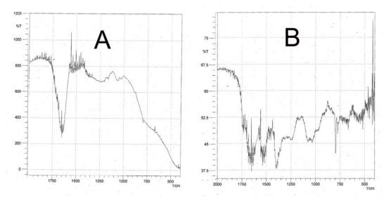
Fig. 5. FTIR spectra of vacuum dried powder of (a) Papaya fruit extract (b) nanoparticles synthesized by 10% fruit extract solution.
