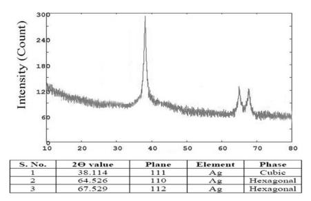
*Fig. 3. XRD pattern of silver nanoparticles synthesized by treating 10% Papaya extract with 1 mM aqueous AgNO*<sub>3</sub> solution.
