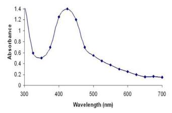
Fig. 2. UV-Vis absorption spectrum of silver nanoparticles synthesized by treating 1mM aqueous AgNO<sub>3</sub> solution with 10% Papaya fruit extract after 5 hrs.
