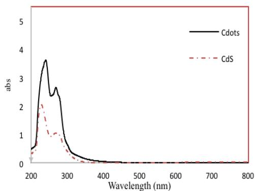
Fig. 4. Results Characterization of Cdot and Carbon dots/Sulfur with UV-Vis.
