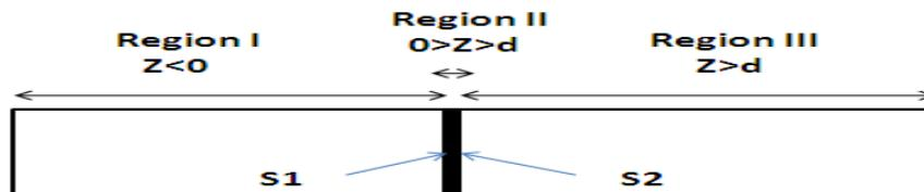
Fig. 1. Rectangular Waveguide Loaded with PVDF-13%LIG Sample
