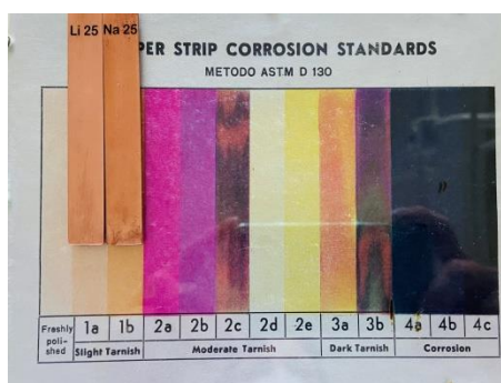
Fig. 1. Corrosion of Li 25 and Na 25 greases
