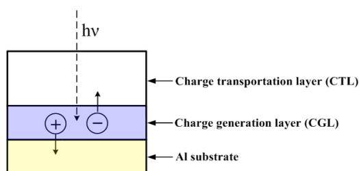
Fig. 2. Configuration of the dual-layer photoreceptor.
