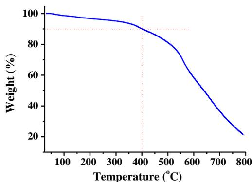
Fig. 6. TGA curve of  $\text{NiPcF}_{16}$ .
