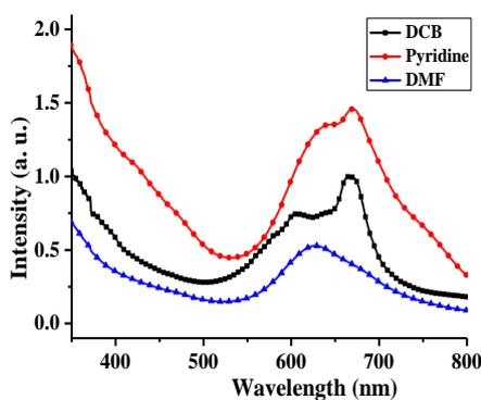
Fig. 3. The UV-vis spectra of NiPcF<sub>16</sub> in different solvents.
