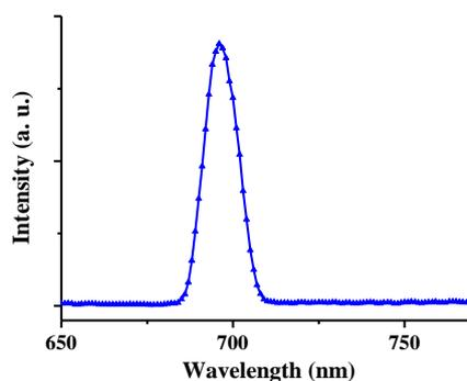
Fig. 4. Fluorescence emission spectrum of NiPcF<sub>16</sub> in DCB.
