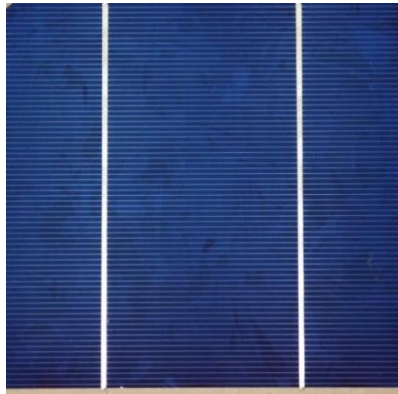
Fig. 1. 156mm by 156mm Polycrystalline solar cell
