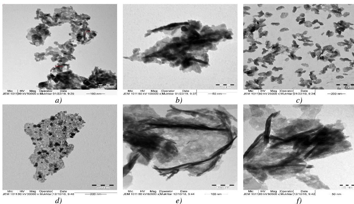
Fig. 2. TEM images of newly fabricated Ni-Co-meso  $\text{MnO}_2$ /Graphene/ $\text{MoS}_2$  (a,b,c, d) compared with Pristine (without Ni and Co addition) sample (e and f).
