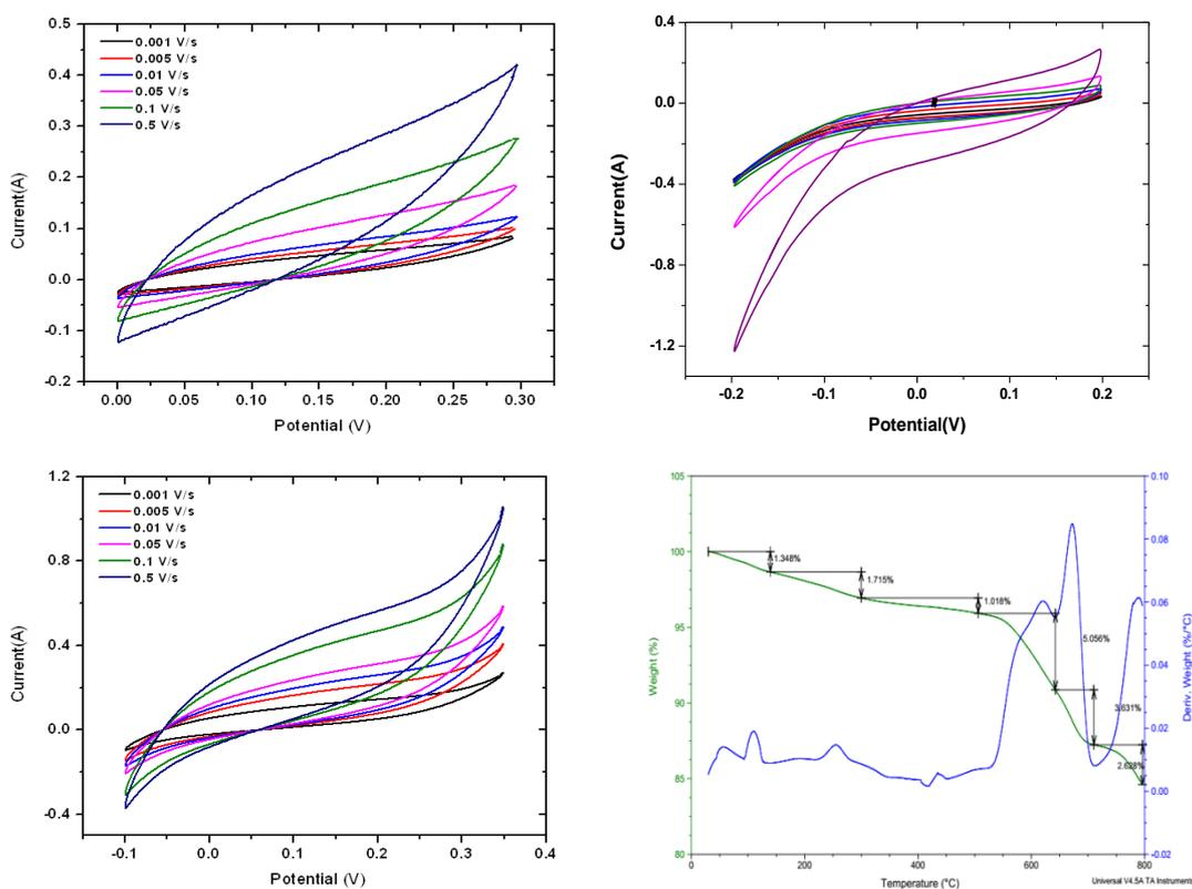
Fig. 3. (a-d) Cyclic voltammetry (CV) and Thermogravimetric analysis (TGA) for modified Ni-Co-meso-MnO<sub>2</sub> catalyst at different scan rates
