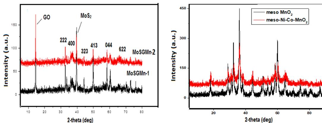
Fig. 1. Comparative XRD images (a) MoS<sub>2</sub>-graphene @meso MnO<sub>x</sub> (MoSGMn-1 & 2) and (b) MoS<sub>2</sub>-graphene@Ni-Co-mesoporous MnO<sub>x</sub>.
