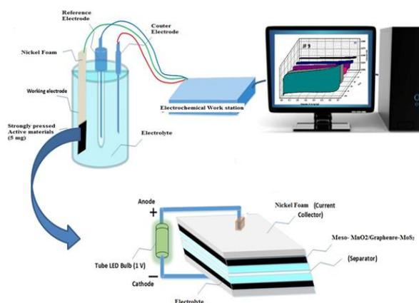
Fig. 4. (a) Schematic of Nickel foam based half cell working electrode setup (b) Our method based Nickel foam design setup for electrochemical analysis
