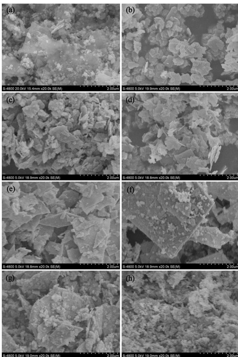
Fig. 2 SEM picture of  $\text{Bi}_2\text{MoO}_6$  catalysts doped with different  $\text{Er}^{3+}$  ratios
