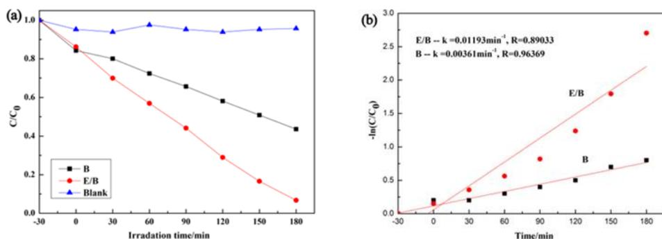
Fig. 6 RhB degradation of B (0% of  $\text{Er}^{3+}$ ) and E/B (0.05% of  $\text{Er}^{3+}$ ) (a) and the dynamics of RhB photodegradation reaction ( $-\ln(C/C_0)$  versus time) for the B (0% of  $\text{Er}^{3+}$ ) and E/B (0.05% of  $\text{Er}^{3+}$ ) (b)
