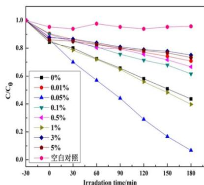
Fig. 3 degradation chart of  $\text{Bi}_2\text{MoO}_6$  catalysts doped with different  $\text{Er}^{3+}$  ratios
