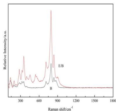
Fig. 4 Raman spectra of B (0% of  $\text{Er}^{3+}$ ) and E/B (0.05% of  $\text{Er}^{3+}$ )
