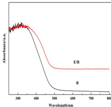
Fig. 5 UV-vis. DRS spectra of B (0% of  $\text{Er}^{3+}$ ) and E/B (0.05% of  $\text{Er}^{3+}$ )
