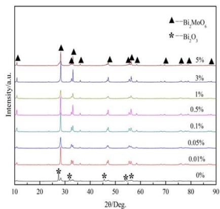
Fig. 1 XRD patterns of  $\text{Bi}_2\text{MoO}_6$  catalysts doped with different  $\text{Er}^{3+}$  ratios
