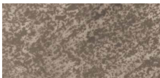
Plate 4: Micrograph of Sample A after 360h in 0.1M HCl
