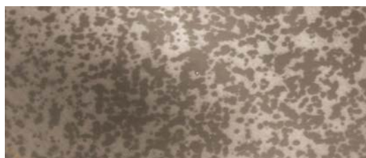
Plate 5: Micrograph of Sample A after 720h in 0.1M HCl
