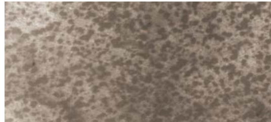
Plate 7: Micrograph of Sample A after 360h in sea water
