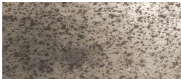
Plate 14: Micrograph of Sample B after 720h in sea water
