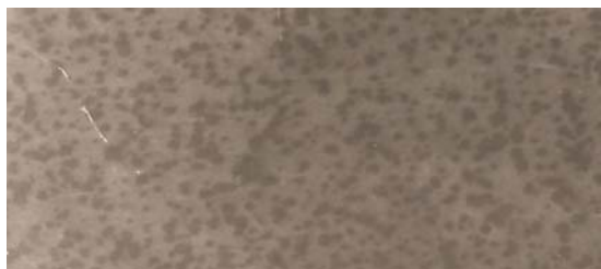
Plate 10: Micrograph of Sample B after 360h in 0.1M HCl
