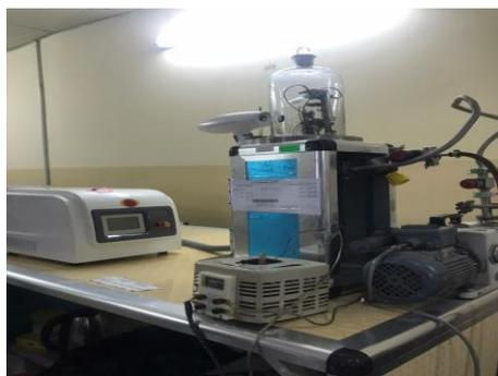
*Fig. 1 the system of the pulse laser deposition (pld)*
