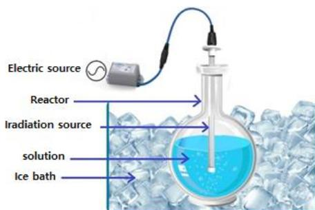
Fig. 1. photo-cell of Synthesis QDs CuS.
