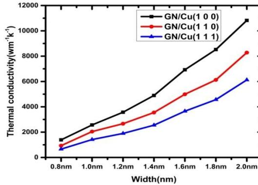
Fig. 6. Thermal conductivity variation of GN/Cu (1 0 0) (black), GN/Cu (1 1 0) (red) and GN/Cu (1 1 1) (blue) as a function of width at 300k temperature with fixed length 10nm.
