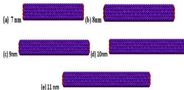
Fig. 3. Schematic atomic structures of GN/Cu nanocomposites with variation in length from 7 nm to 11 nm with a fixed width of 10 nm.
