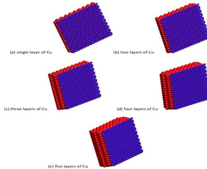
Fig. 7. Graphene copper nanocomposites with copper layers at the bottom (a) single layer of Cu (b) two layers of Cu (c) three layers of Cu (d) four layers of Cu (e) five layers of Cu with red color and graphene with violet color on top of the copper.
