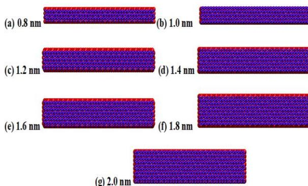
Fig. 5. Schematic atomic structures of GN/Cu composites with variation in width from 0.8 nm to 2.0 nm with fixed length 10 nm.
