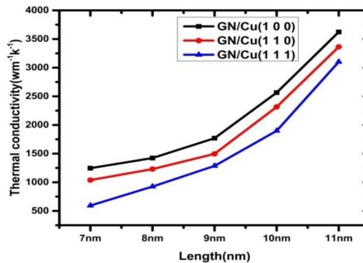
Fig. 4. Thermal conductivity variation of GN/Cu (1 0 0) (black), GN/Cu (1 1 0) (red) and GN/Cu (1 1 1) (blue) as a function of length at 300k temperature with fixed width 10nm.
