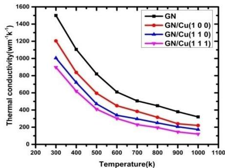
Fig.2. Thermal conductivity of GN (black), GN/Cu (1 0 0) (red), GN/Cu (1 1 0) (blue) and GN/Cu (1 1 1) (pink) as a function of temperature.
