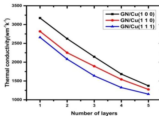
Fig. 8. Thermal conductivity variation of GN/Cu (1 0 0), GN/Cu (1 1 0), and GN/Cu (1 1 1) as a function of the number of copper layers from 1 to 5.
