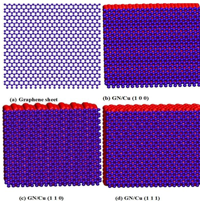
*Fig.1. Schematic presentation of simulation model (a) Graphene sheet (b) GN/Cu (1 0 0) (c) GN/Cu (1 1 0) and GN/Cu (1 1 1).*
