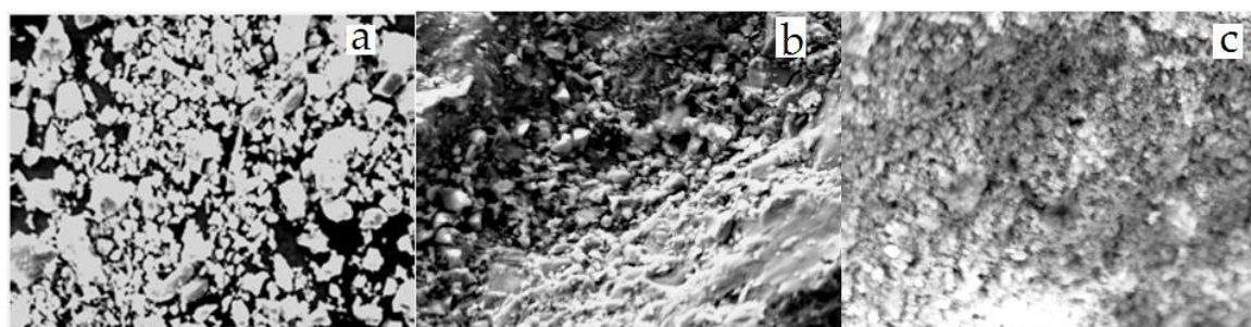
Fig. 1. SEM images of a) Fe 0 b) CMC-Fe 0 c) CMC-Fe 0 /Ag nanoparticles.
