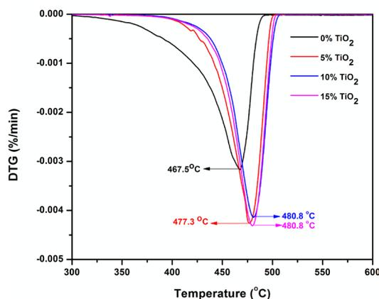
Fig. 5. DTG curves of  $\text{TiO}_2/\text{LDPE}$  nanocomposites films.
