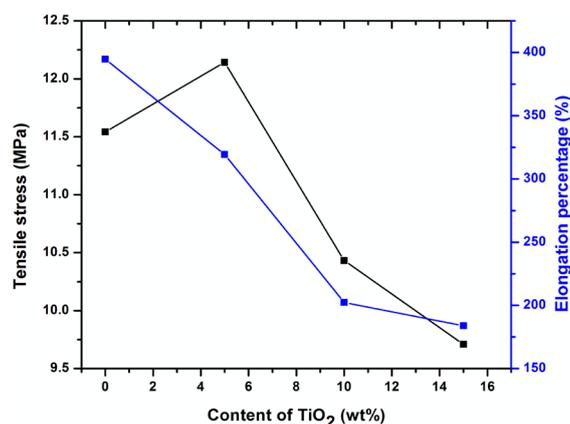
Fig. 6. Combination of strength and elongation versus the content of  $\text{TiO}_2$  nanoparticles.
