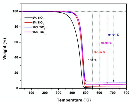
Fig. 4. TGA curves of TiO<sub>2</sub>/LDPE nanocomposites films.
