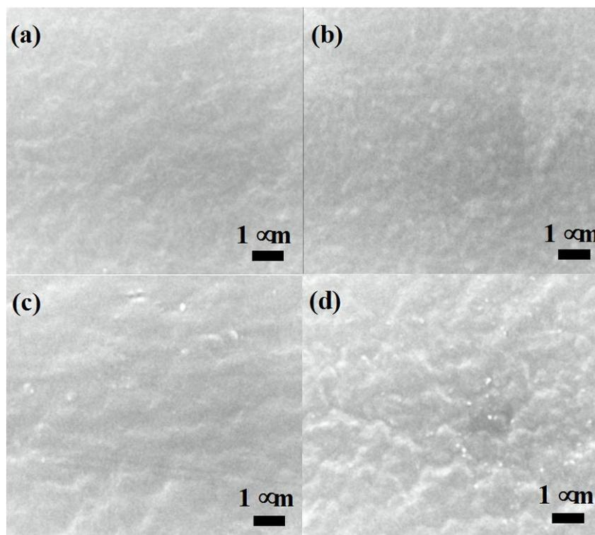
Fig. 1. SEM image of surface morphology of TiO<sub>2</sub>/LDPE nanocomposites films containing different contents of TiO<sub>2</sub> nanoparticles (a) 0 %wt, (b) 5w%wt, (c) 10 %wt and (d) 15 %wt.
