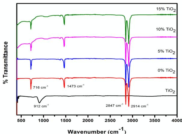
Fig. 3. FTIR spectra of TiO<sub>2</sub>/LDPE nanocomposites films.
