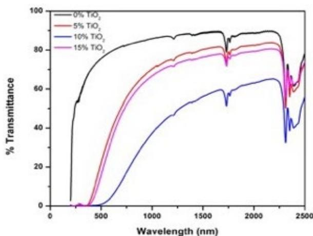
Fig. 2. Transmittance spectra of TiO<sub>2</sub>/LDPE nanocomposites films.
