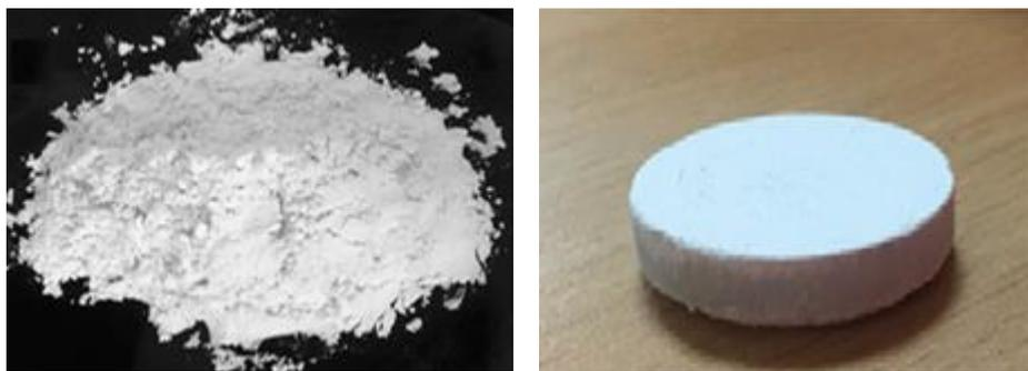
Fig. 1. a- the powder of lithium niobate LiNbO<sub>3</sub>. b- The target before the annealing process.
