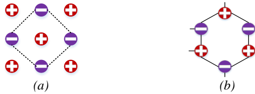
Fig. 5. (a) Centrosymmetric crystal having center of symmetry (b) Non-Centro-symmetric crystal having no center of symmetry [8].
