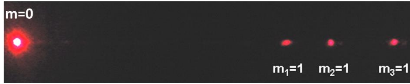
Fig. 4. Diffraction pattern from a structure composed of superimposed gratings with \Lambda_1=1.1 \mu\text{m} , \Lambda_2=1 \mu\text{m} and \Lambda_3=0.9 \mu\text{m} formed in As_2S_3 film
