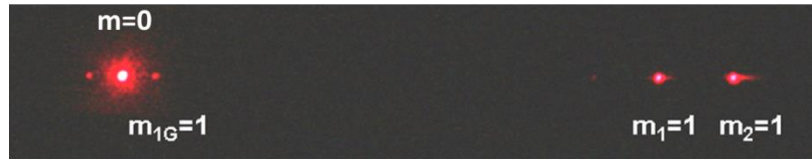
Fig. 2. Diffraction pattern from a structure composed of superimposed gratings with \Lambda_1=1 \mu\text{m} and \Lambda_2=0.92 \mu\text{m} formed in \text{As}_2\text{S}_3 film
