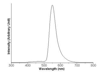
Fig. 3 PL emission of CdTe synthesized by the 200 °C and 72 h solvothermal reaction
