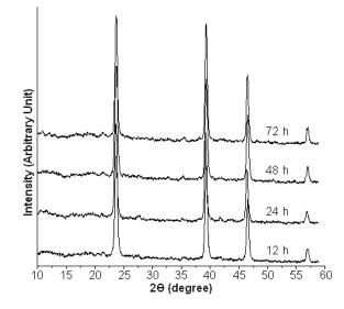
Fig. 1 XRD patterns of CdTe samples synthesized by the solvothermal reaction at 200 °C for 12, 24, 48 and 72 h
