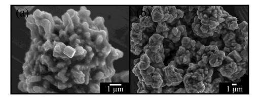
Fig. 2 SEM images of CdTe samples synthesized by the solvothermal reaction at 200 °C for (a) 12 h and (b) 72 h.
