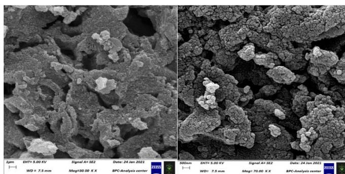
Fig. 3. SEM images of GO/Ag nanocomposite.
