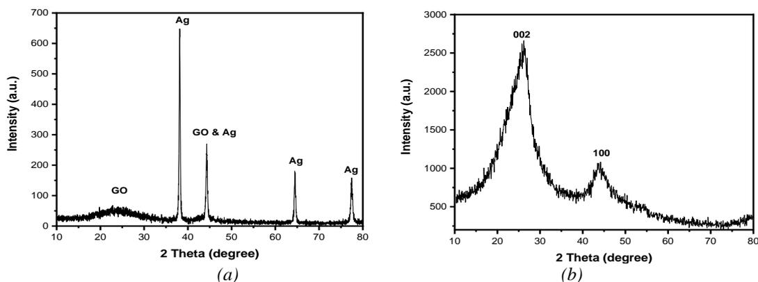
Fig.6. XRD of a) GO Nano-sheets and, b) GO-Ag nanocomposites.
