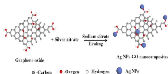
Fig. 1. Synthesis of GO /Ag nanocomposites [47].
