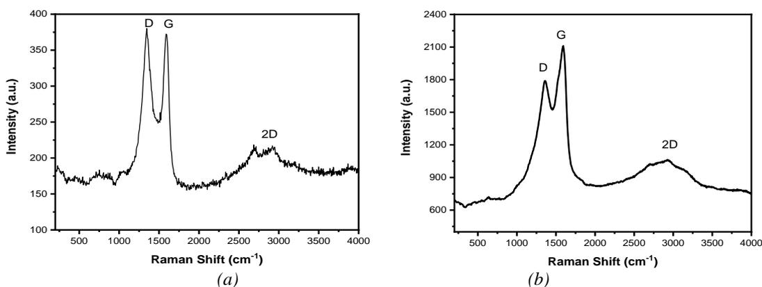
Fig.7. Raman spectra of a) GO nano-sheets and, b) GO-Ag nanocomposites.
