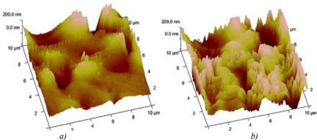
Fig. 4. AFM analysis of a) Pr/PLA and b) Pr/PLA/HA.
