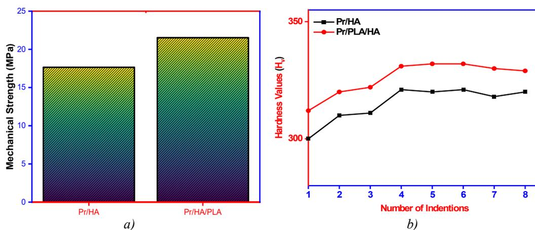
Fig. 5. Mechanical strength and Vickers Micro-hardness Evaluation of a) Pr/PLA and b) Pr/PLA/HA.
