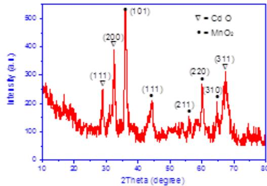
Fig. 1. XRD pattern of CdO-MnO<sub>2</sub> nanoparticles.
