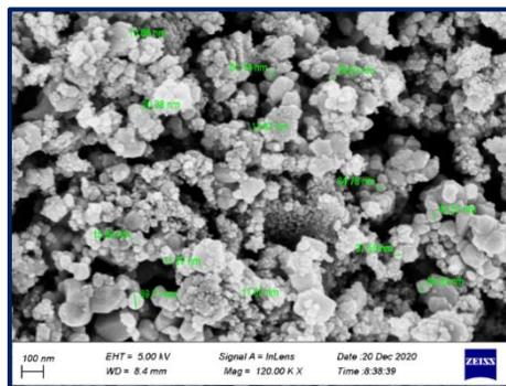
Fig. 2. FE-SEM image CdO-MnO<sub>2</sub> nanoparticles.
