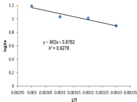
Fig. 4. The relation between  $\log X_e$  and  $1/T$  for the adsorption of MO.
