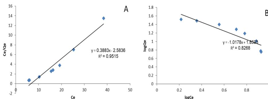
Fig. 3. Adsorption equation of (A) as Langmuir isotherm, (B) Freundlich isotherm, at 298 K.
