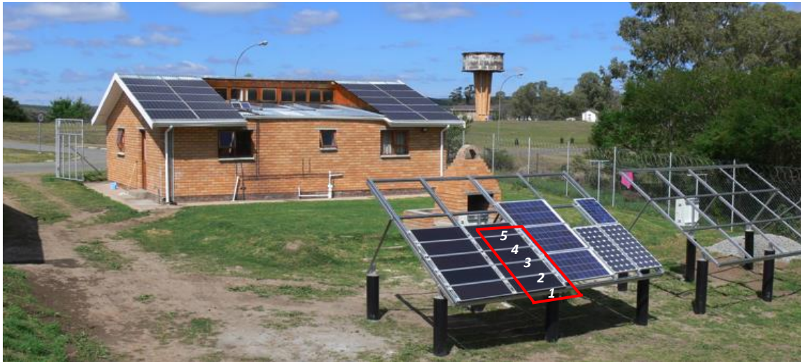
Fig. 2: Outdoor monitoring of different PV modules on the rack, the red link indicate the investigating modules
