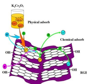
Fig. 10. Adsorption mechanism of graphene hydrogel on Cr (VI).
