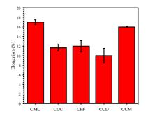
Fig. 8. Elongation measurement results (%) on various nanofiber membranes.
