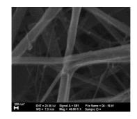
Fig. 5. Cross section formed by the addition of citric acid crosslink agent.
