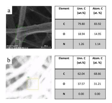
Fig. 6. SEM EDX results (a) section of cross section and (b) non cross-section.
