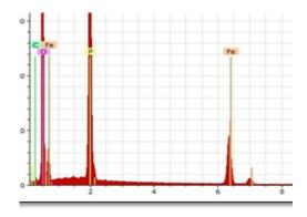
Fig. 5.EDX spectrum for LiFePO<sub>4</sub>/C.
