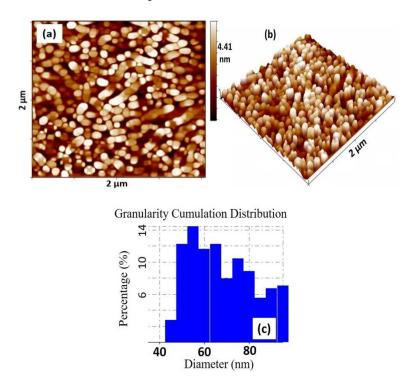
Fig. 3.AFM micrograph for LiFePO $_4$  (a) 2D (b) 3D and (c) Granularity cumulation distribution chart.
