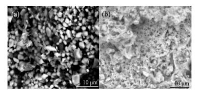
Fig. 2. SEM images of (a) LiFePO<sub>4</sub> and (b) LiFePO<sub>4</sub>/C.
