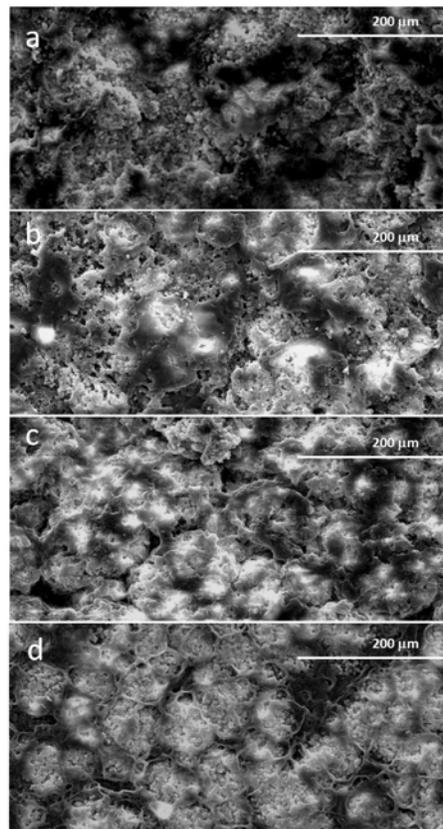
*Fig.3. SEM images of the cross-section of Cas-PHEMA hybrids with decreasing Cas content: a - A, b - C, c - D, d-E.*
