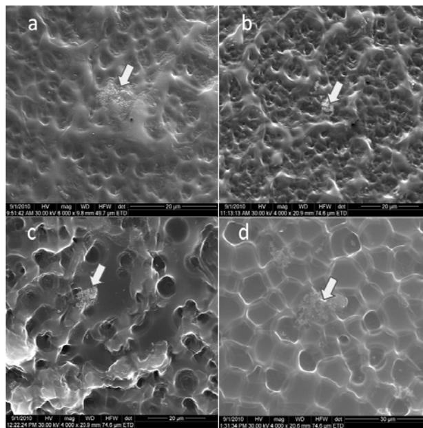
Fig.6. SEM images presenting PHEMA surfaces (a-A0, b-B0, c-C0 and d – E0) after the incubation in SBF. Calcified small areas (indicated by white arrows) are accidentally observed.
