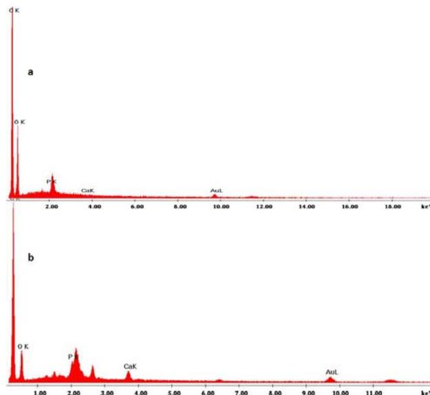
Fig.8. EDAX spectra indicating the presence of P before (a) and after (b) the SBF incubation of sample C. Ca is detected only after the SBF treatment (b) thus proving the successful *in vitro* calcification.
