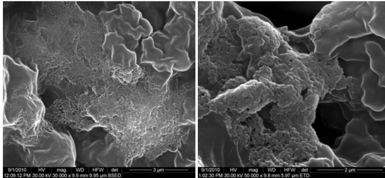
Fig.7. SEM images showing mineral nucleation areas formed on sample C (left) and E (right) after 14 days incubation in SBF.
