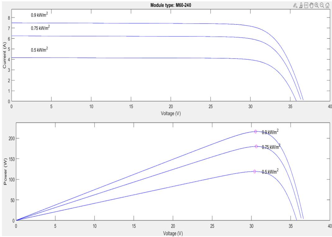
*Fig. 2. Characteristic Curves of M60-240 under Different Irradiance at 25 °C.*
