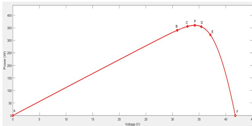
Fig. 13. The P-U characteristic curve of PV.
