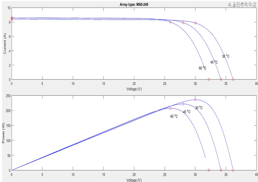
Fig. 3. Characteristic Curves of M60-240 at Different Temperatures under  $1000\text{W}/\text{m}^2$ .
