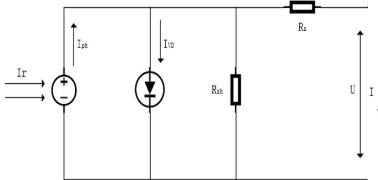
Fig. 1. Equivalent Circuit of Photovoltaic Cell.
