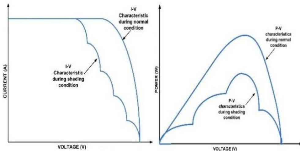
Fig. 4. Characteristic curves under partial shading conditions.
