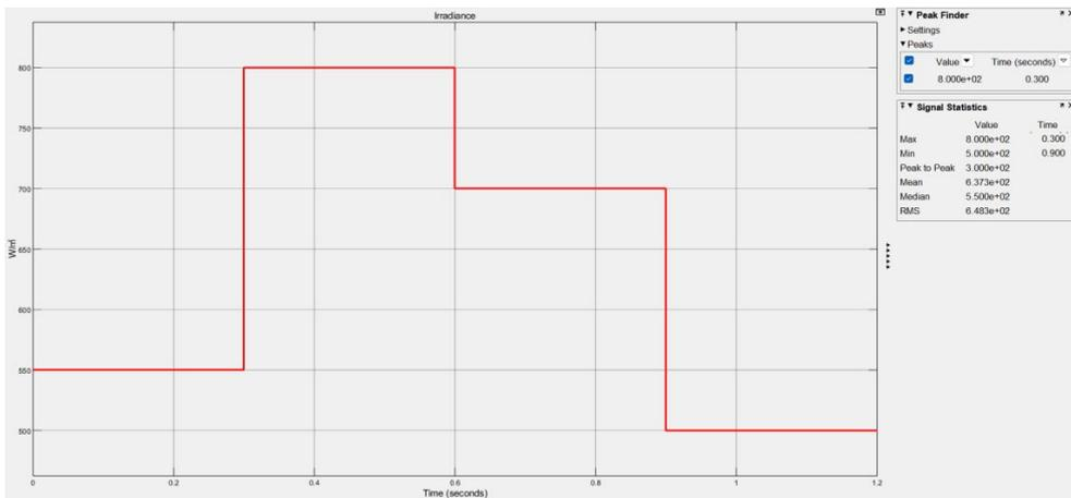
Figure 16 c) The Varied Irradiation and Temperature in the Simulation Module Varied Irradiation\_PV Array2
