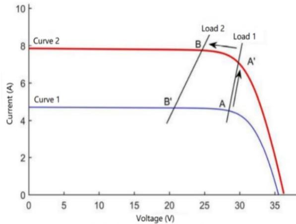
Fig. 6. Schematic Diagram of MPPT.
