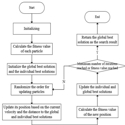
Fig. 7. The Flowchart of the Async-PSO Algorithm.
