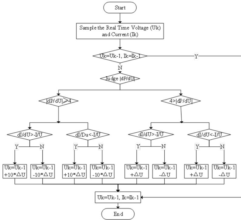
Fig. 12. The Flowchart of Variable Step-Size INC Method.
