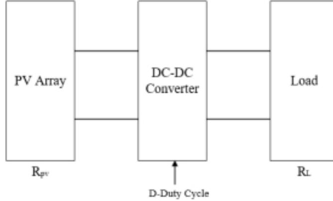
Fig. 5. Connecting Diagram of DC-DC Converter.
