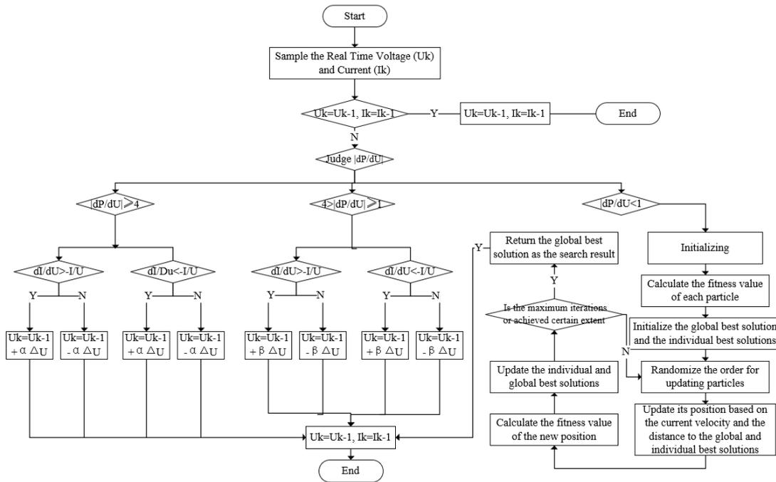
Fig. 14. The Flowchart of Async-PSO and VSINC Algorithm.
