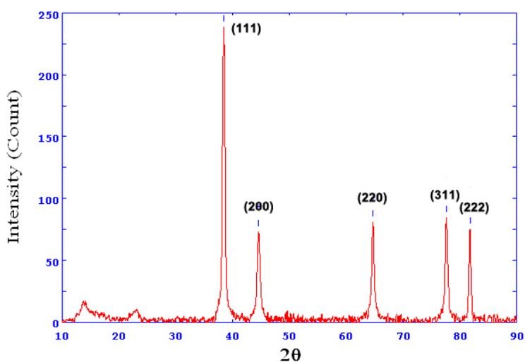
Fig. 2. X-ray diffraction pattern of Ag NPs at room temperature synthesized by Capsicum fruits extract with  $\text{AgNO}_3$  solution.
