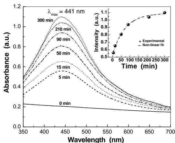
Fig. 3. UV-vis spectra for Ag NPs recorded as function of time of reaction of 0.25M aqueous solution of  $\text{AgNO}_3$  with *Capsicum* fruits extract. Inset: Absorbance at  $\lambda_{\text{max}}$  ( $\xi$ ) as a function of time with theoretical fit Eq.(1).
