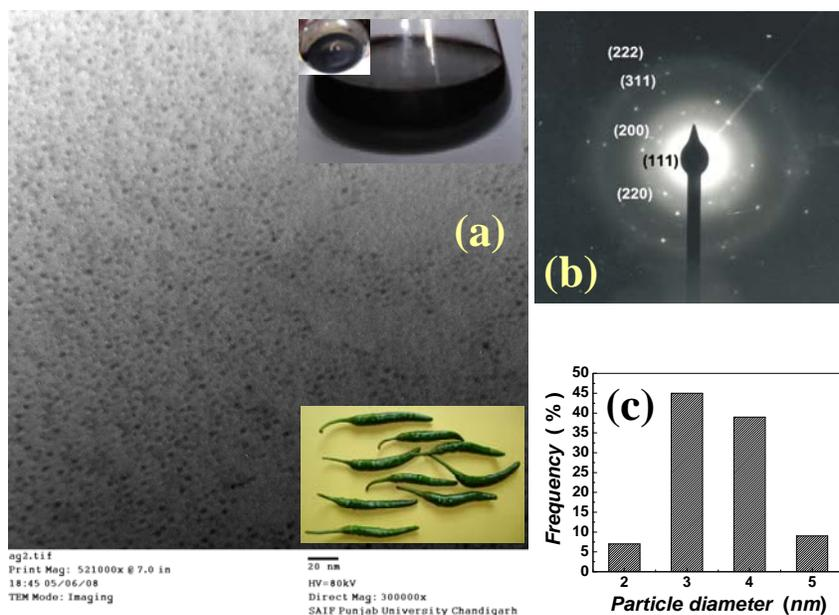
Fig. 1. (a) TEM image of Ag NPs synthesized by reduction of  $\text{Ag}^+$  ions using Capsicum fruits extract, Insets: Ag NPs in medium, deposition of Ag NPs (bottom view) and Capsicum fruits, (b) SAED pattern and (c) particle size distribution (%) of Ag NPs.
