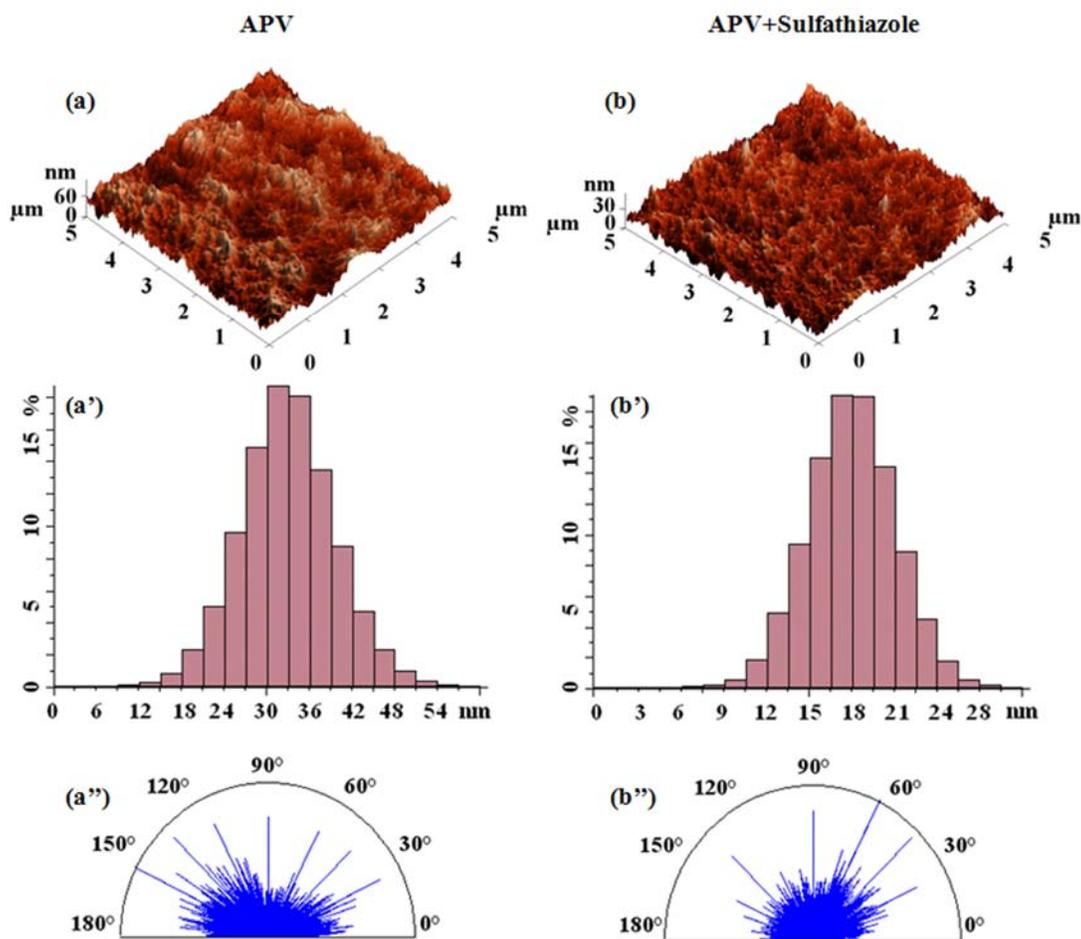
Fig.4 Three-dimensional tapping mode AFM height images (a, b), height histograms (a', b') and angular spectra (a'', b'') for APV and APV + sulfathiazole samples
