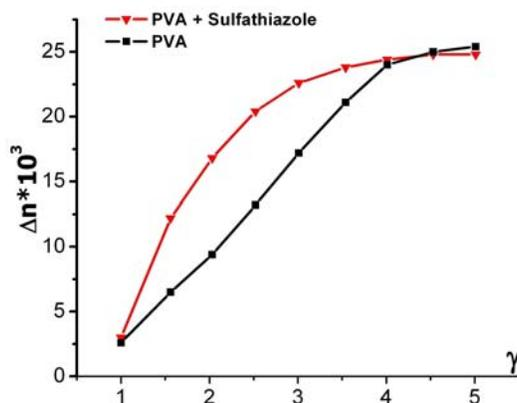
Fig.3 Birefringence vs. degree of stretching for a) pure PVA and b) PVA+ sulfathiazole films
