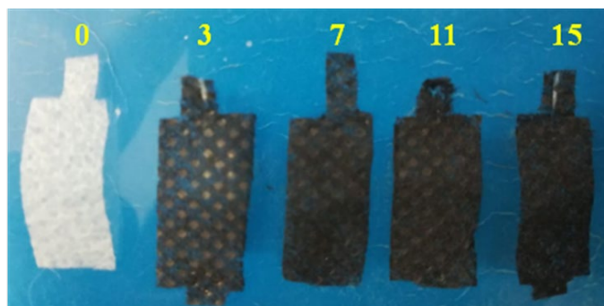
Fig. 3. Dip coating method prepared non-woven paper materials at different coating time (P0-P4).
